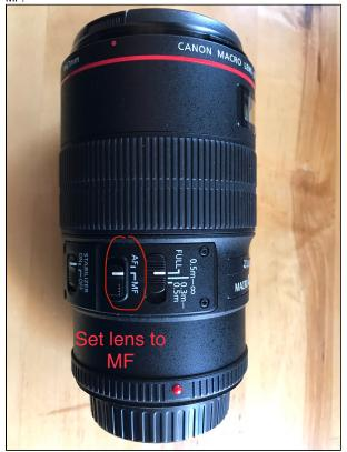
When in auto-focus, the camera is supposed to focus when the focus signal is triggered, but in some cases the internal focus is not fast enough to finish by the time the shutter signal comes and the camera won't fire if the focus is not finished. To eliminate the need for focus, set the camera to manual and now the camera will only listen to the release command. When shutting in shutter release mode, the camera should always be in manual focus.
