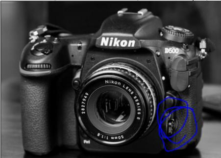
For these cases, please flip the camera switch to MF, to make sure you are shooting in manual mode and that focus setting issues do not interfere with the shutter release issues.
